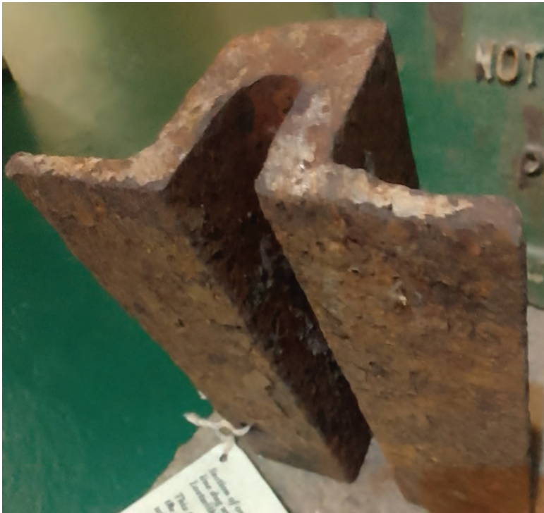
Plate 5: A piece of bridge-rail as used in the laying of the Mallow-Tralee railway line (Source: Courtesy Bodmin Town Museum, Cornwall).
